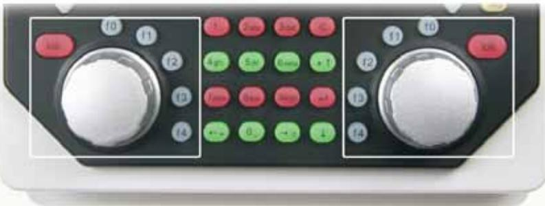
Each control desk consists of the throttle control knob for changing locomotive speed and driving direction as well as of the f0 to f4 special function keys. The [lok]-key on each control desk serves to select new locomotives on the controller.
